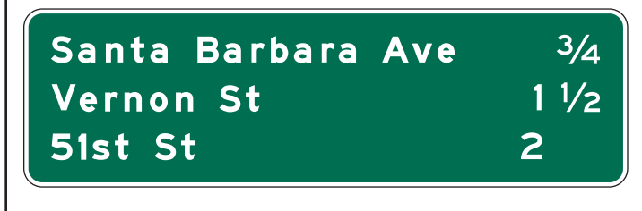
Figure 2E-31. Interchange Sequence Sign
