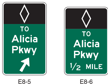
Figure 2G-11. Examples of Barrier-Mounted Guide Signs for an Intermediate Egress from Preferential Lanes
